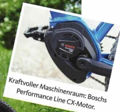
Kraftvoller Maschinenraum: Bosch Performance Line CX-Motor.
